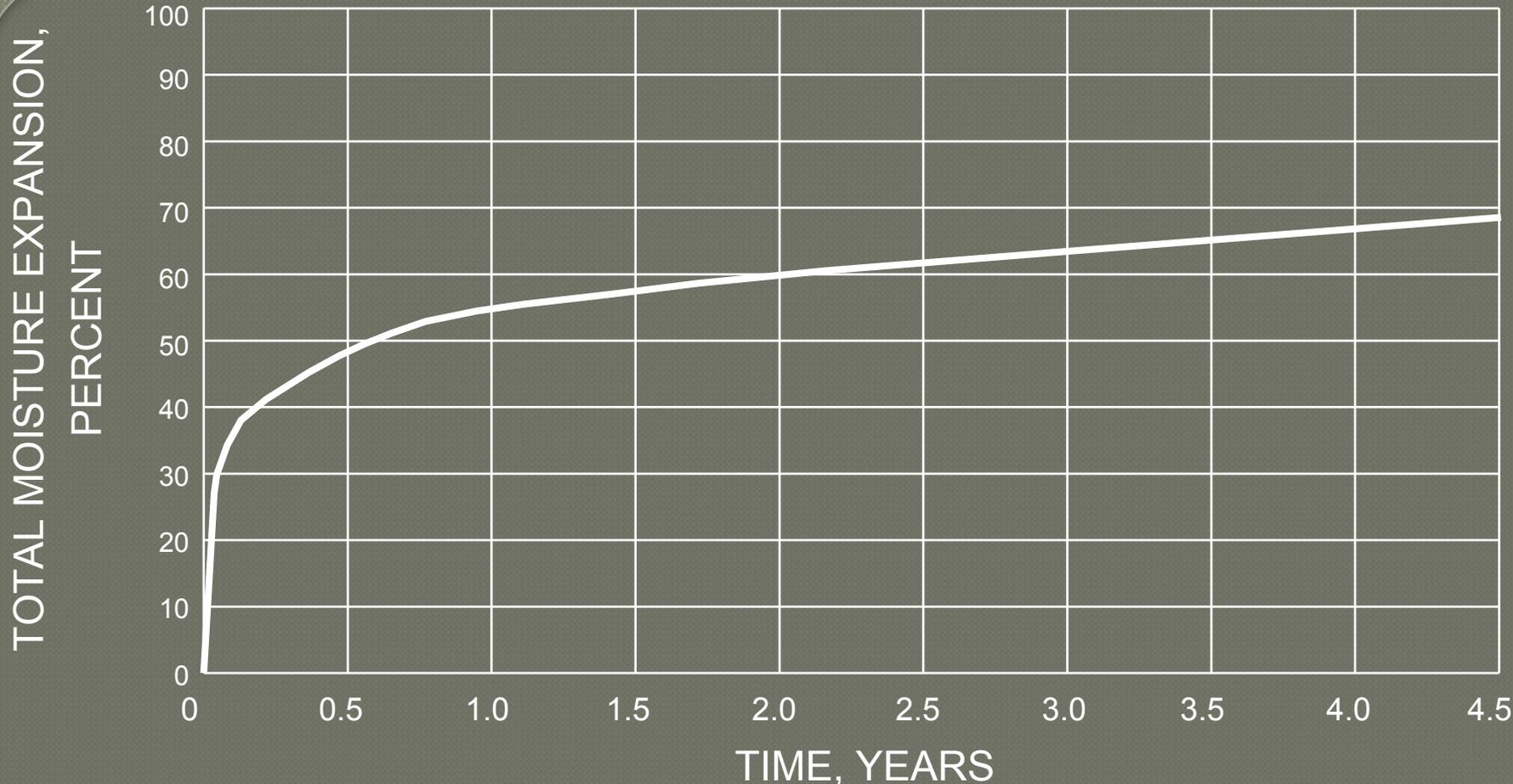
Moisture Expansion of Fired Clay Brick vs. Time Fig. 1
