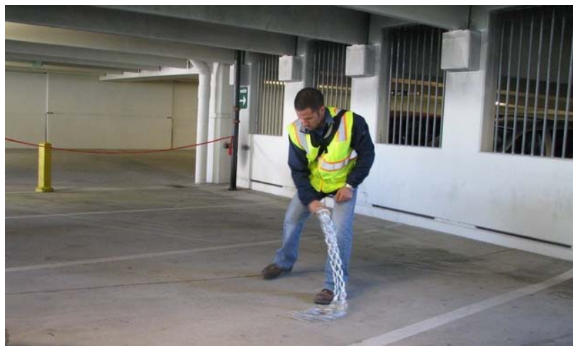
Figure 2.2.1 Testing for delamination using Chain Dragging
