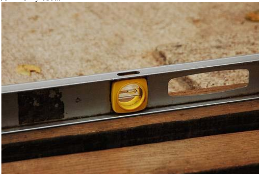
Figure 2.1.1 Carpenter level showing body, insert, vial, and cutouts
