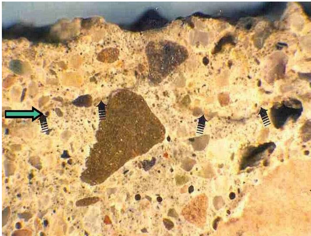
Figure 2.17.4 Poor curing caused by a "Leisegang Ring" type feature in concrete (arrows)
