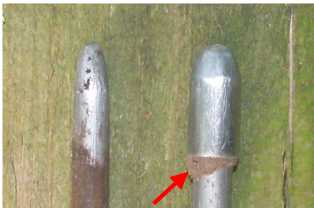
Figure 2.8.2 Ground Probe tips with upset tip with the clay return (arrow)
