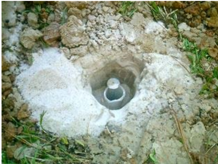
Figure 2.6.2 Example of a 35-ft deep benchmark
