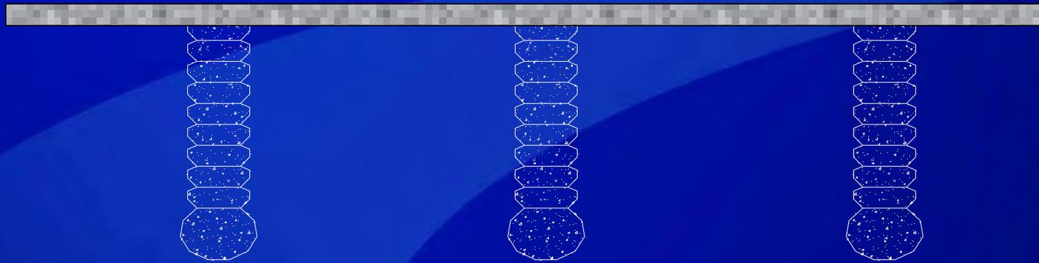
**Elements reinforce soft and compressible soils for support of relatively thin floor slabs.**
