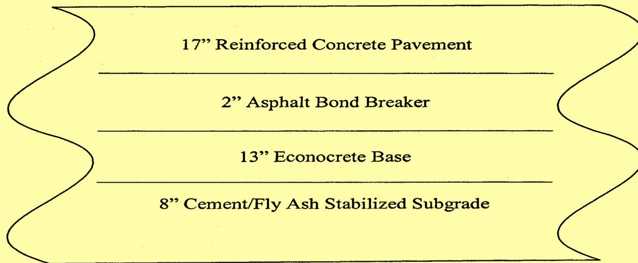
Figure 4: Runway and Taxiway Pavement Cross-Section
