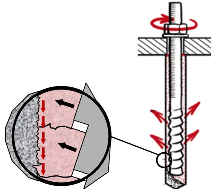
**Special design of helix and expansion forces means that cleaning is not required**
