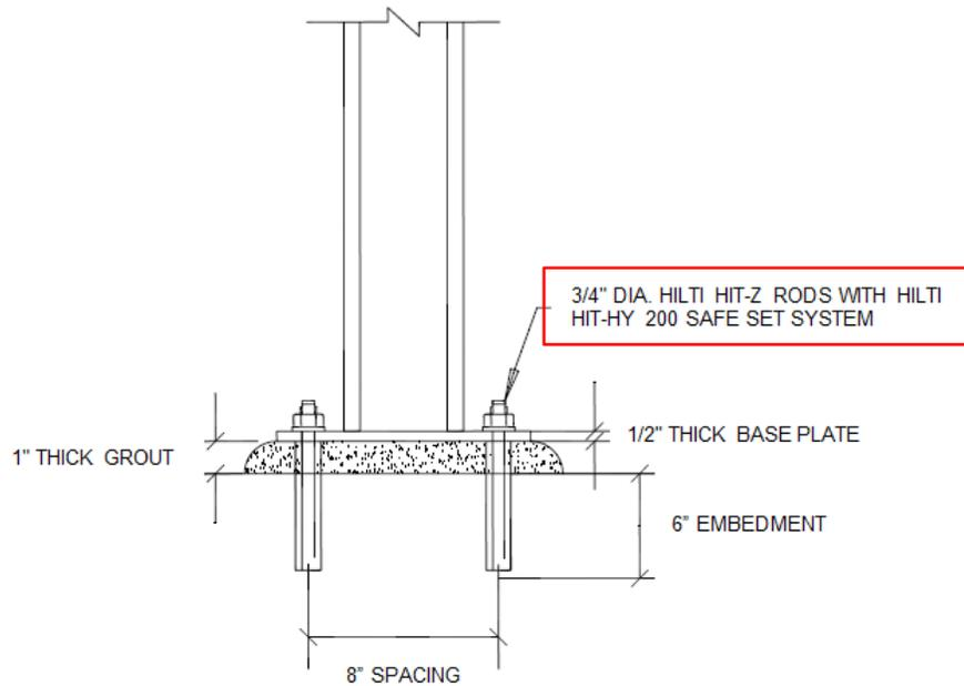
2 COLUMN BASE PLATE ATTACHMENT TO CONCRETE
