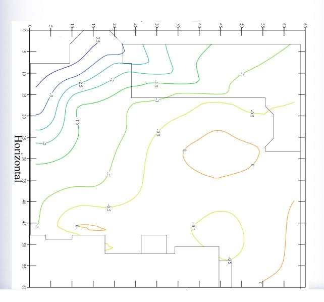
Areas of the contour that are outside the floor plan can be filled by pasting white filled areas using excel drawing tools, or group pictures and edit in "Paint" what ever is easiest
